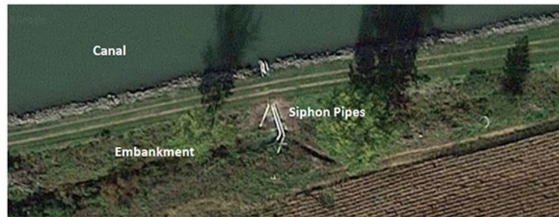
Siphon (n): a bent pipe that carries water upward over an obstruction and then back downwards
